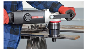
Steel plate beveling
