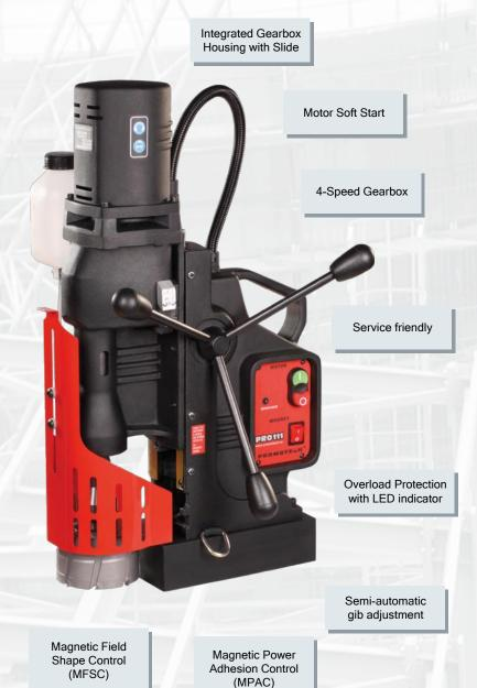
PRO 111 is equipped with electromagnetic base featuring magnetic field shape control system (MFSC) and magnetic power adhesion control module (MPAC), which detects adhesive force of electromagnetic base and protects both the machine and the operator from work on too thin workpieces.
